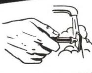
4. CLEAN BLADE in razor by loosening handle, then rinsing in hot water and shaking. Wiping the blade is likely to damage the edges
